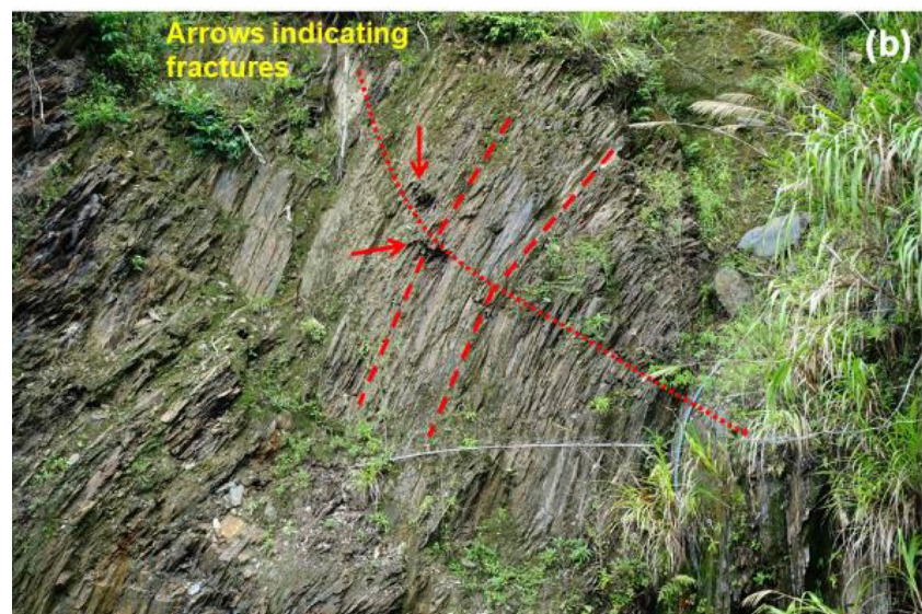
(b) Fractures in the rock layers (zoomed-in view of the box in (a))
